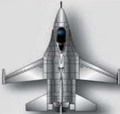
Tapered leading edge, straight trailing edge
