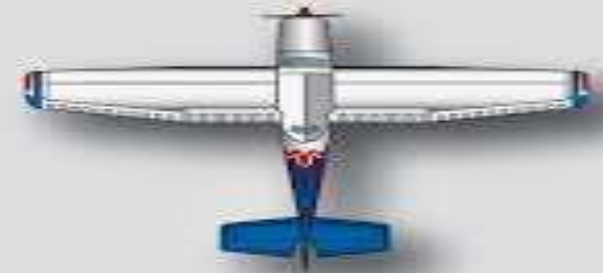
Straight leading edge, tapered trailing edge
